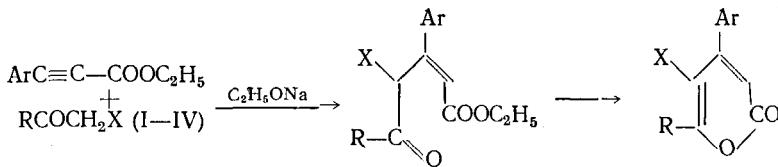
(I) X=C<sub>6</sub>H<sub>5</sub>; (II) R=Ar, X=OR'; (III) X=COOC<sub>2</sub>H<sub>5</sub>; (IV) X=COR'
